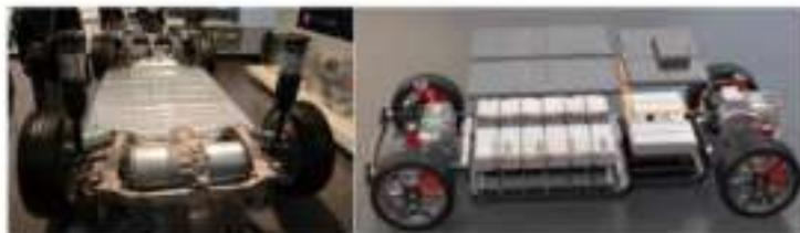
Figure 3 - Examples of the positioning of the battery packs in EVs, which is found in the streets.
