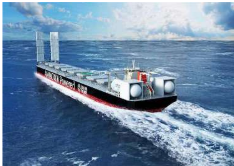
Computer generated image of the 210,000 dt ammonia-fuelled bulk carrier.
