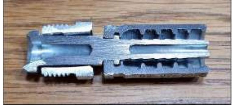
*Section through blocked CO<sub>2</sub> pilot hose coupling showing incomplete bore through the stem.*
