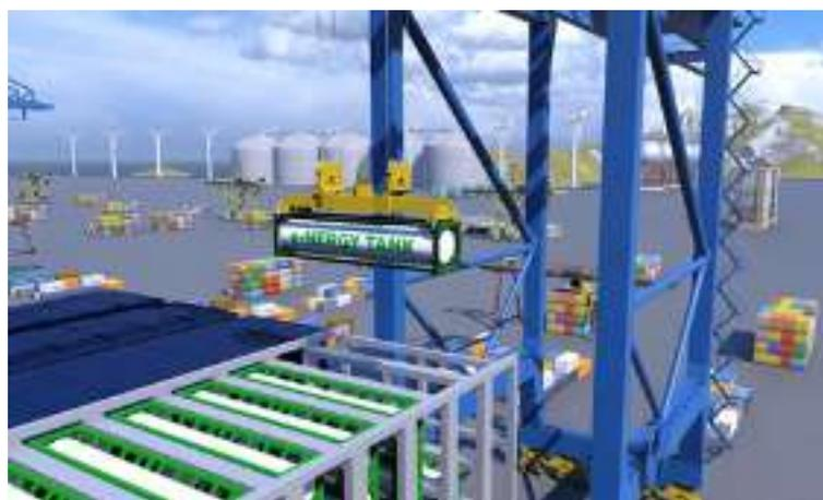
Since LNG containers are portable, the total number of containers can be easily optimised according to the owners' requirements. Simple and easy to install on board, when a ship is in port, the empty containers can be taken out and replaced by filled ones.
