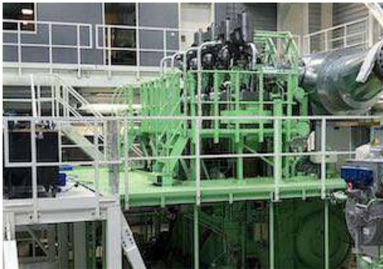
MAN engine testbed.
