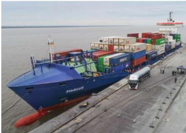
Measurements were carried out on a voyage between Brunsbüttel, Germany and Rotterdam, with SNG comprising approximately 50% of the bunkered gas at 85% engine load. *ElbBLUE* is powered by an MAN 51/60DF four-stroke engine. As a multi-fuel engine, the unit allows operation with either HFO or liquid natural gas (LNG) as fuel. The ship's test-run proved that the latter can be replaced by SNG without engine modification.
