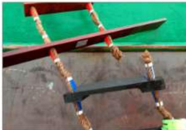
Figure 2: Example of a failed pilot ladder
