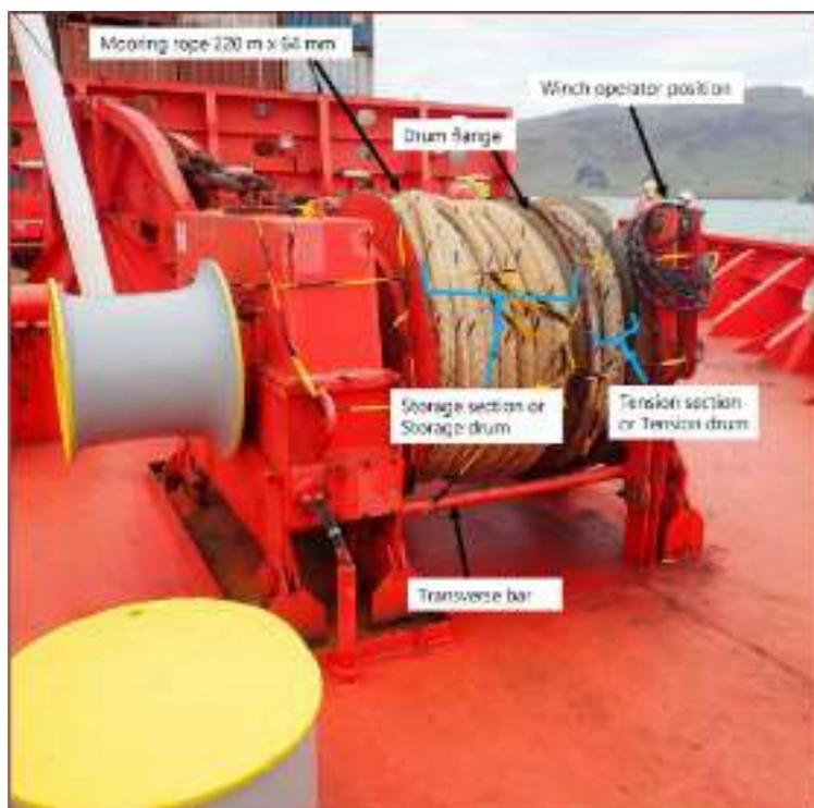
View of winch shows the rope handler would be unable to see the winch operator. A transverse bar was fitted for rigidity during travel for installation. A safety improvement would be to remove the bar after installation.
