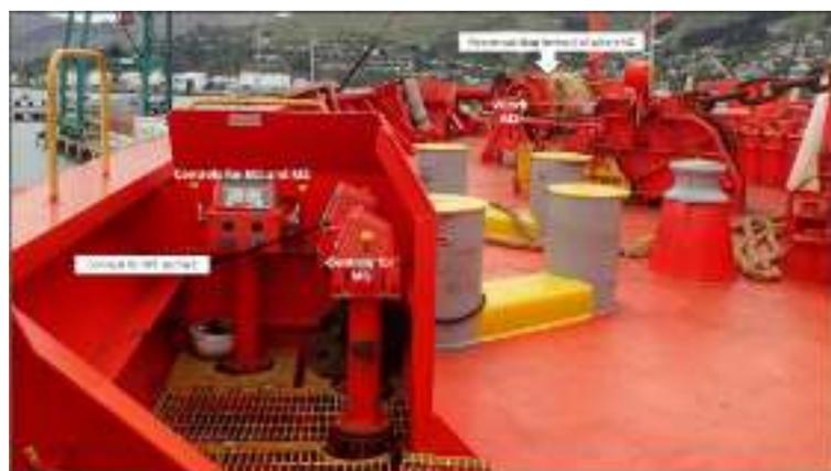
The port half of the forward mooring deck. Winch operator console is in left foreground. The large mooring winch is in the distance. Shows how the winch operator would have lacked a clear view of the rope handler - who was working on the other side of the winch.
